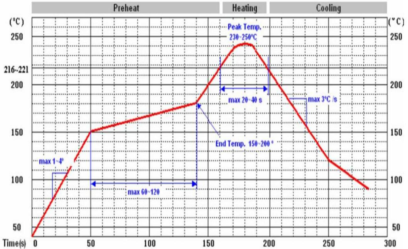
**Note:** The final soldering temperature chosen at the factory depends on additional external factors like choice of soldering paste, size, thickness and properties of the baseboard, etc. Exceeding the maximum soldering temperature in the recommended soldering profile may permanently damage the module.
